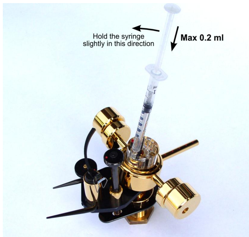
Fig. 9. Damping of the vertical mode of motion. Inject max. 0.2 ml. Not always an advantage.
